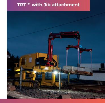
The TRT™ removes and installs all profiles of rail and any gauge of track. Multiple TRTs can be used to move long lengths of rail as well as transport, remove and install associated iron work like switches and crossings. The product has full acceptance to operate in the UK, Australia, New Zealand, Malaysia and North America.
